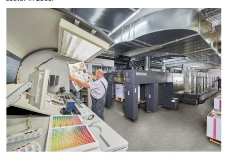
Eltosch Grafix, the sheet-fed expert in the Hönle Group and OEM partner for manroland sheetfed, optimized and adapted the press to customers' specification. In order to cope with the demands of the print buyers for ecological and attractive print products the existing dryer was converted with two LEC UV modules which produce energy optimized and ozone free .
